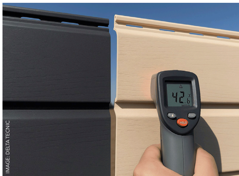
Above: Delta Tecnic says its cool pigments can reduce thermal increase in sun-exposed plastics by up to 30%
